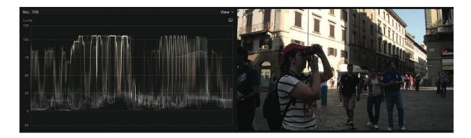
Figure 9.3 Waveform and image.
